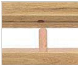
Solid dowel joint
