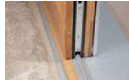
FIBREGLASS THRESHOLD fibreglass threshold with thermally insulated inserts with 5 mm running rail and with a threshold levelling plate allowing almost perfect leveling of the floor inside and outside the house, threshold width 240 mm height 42 mm.
