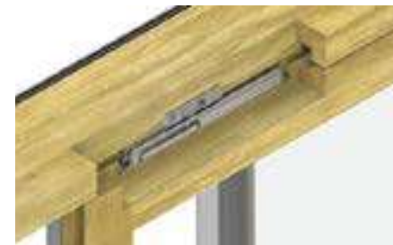
optionally COMFORT STOP SASH DAMPER brakes the sash during opening and closing just before the end position and gently stops it.
