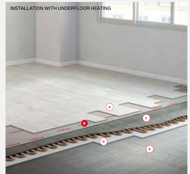
A FINFLOOR B FINFLOOR SILENT ELITE UNDERLAY C UNDERFLOOR HEATING D INSULATION E SUB-FLOOR
